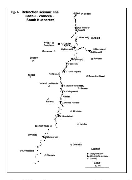
Gravity, magnetics and high precision leveling are represented along the refraction profile to create a state of the art geophysical image in the area and to help interpretation and the construction of an improved crustal model of the region crossed by the refraction profile.
