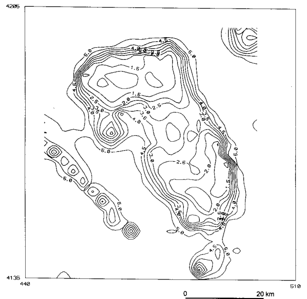
FIG. 10. Gravity model of the Konya anomaly. The model is presented as contours on top of the model. The contour interval is 0.5 km. The density contrast is 0.5 \text{ g/cm}^3 . Edge effects in a narrow band are suppressed in the west, north and east.
