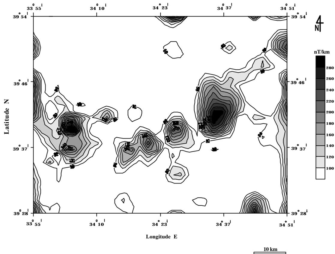
**FIG. 10:** The analytic signal of reduced to the pole anomalies shown in Figure 9.
