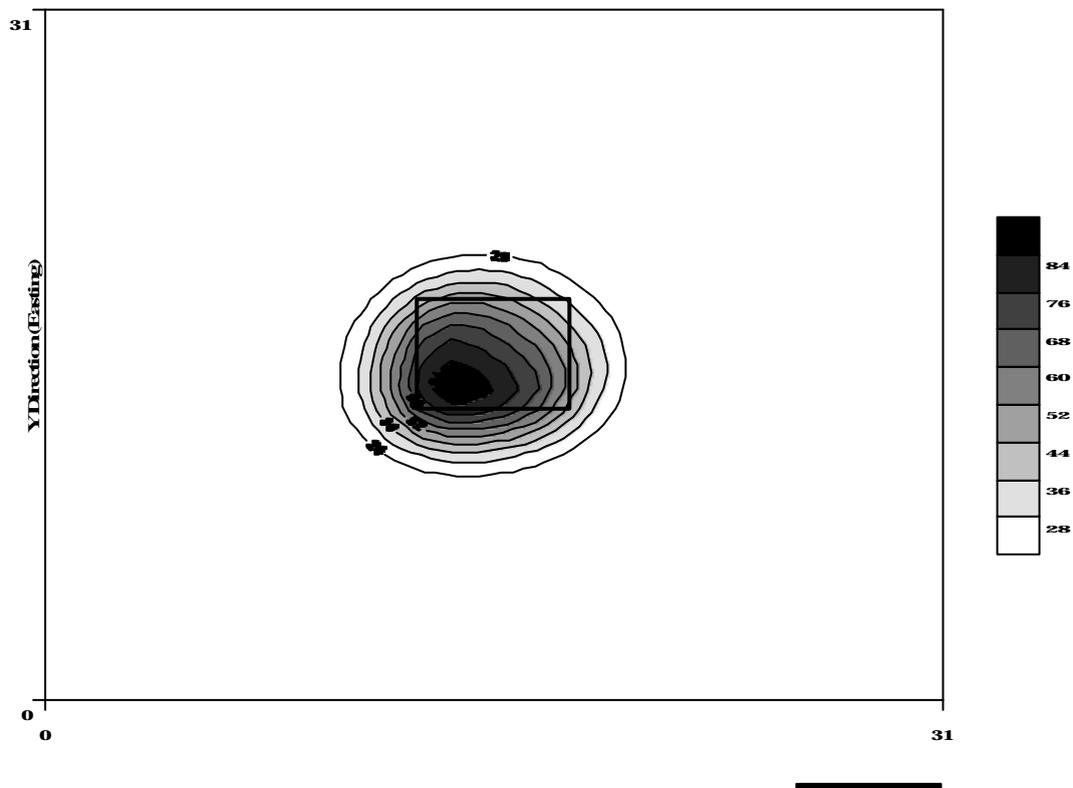
**FIG. 3:** The analytic signal of the magnetic anomaly of Figure 2. Bold lines show plan view of the causative body.
