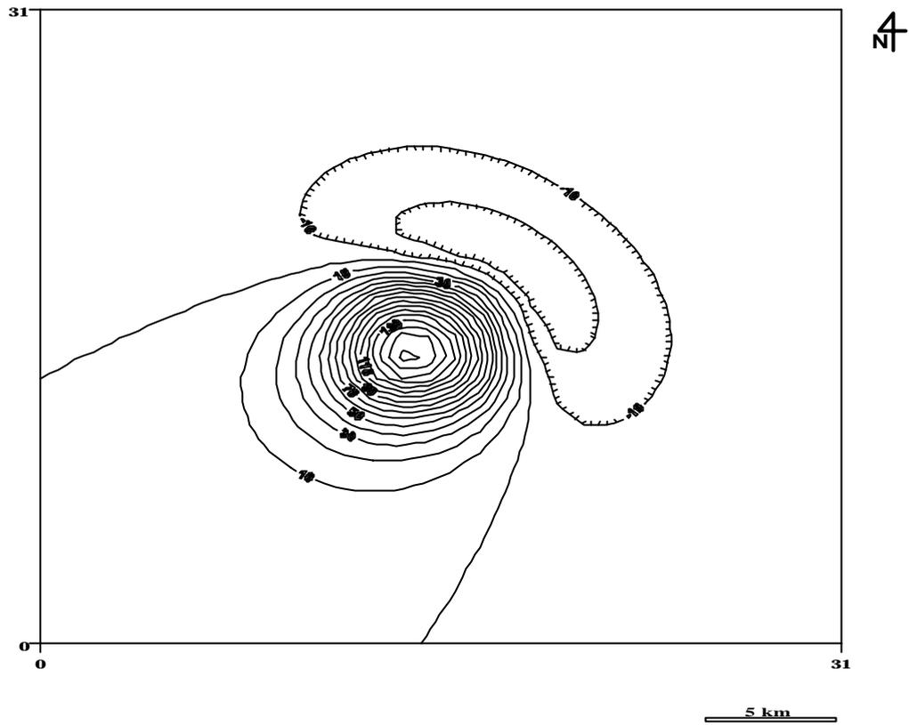
**FIG. 2:** Magnetic anomaly (nT) of the prism model shown in Figure 1. Contour interval is 10 nT.
