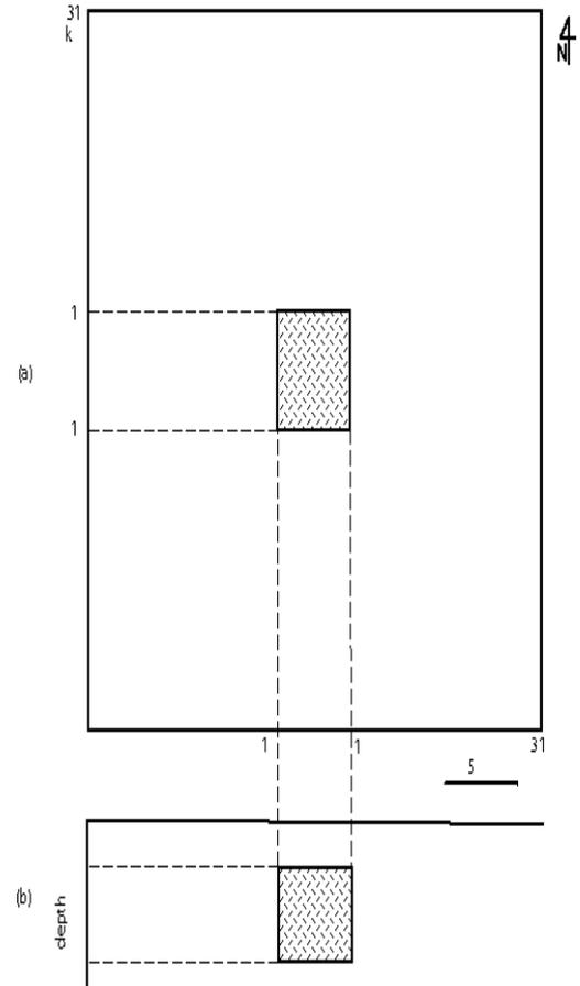
**FIG. 1:** Model (A-plan view, B-section) used to produce magnetic anomalies. The dimensions are  $5 \times 5 \times 4$  km and the burial depth of the upper surface is 2 km. The intensity of magnetization (J) =  $1 \text{ Am}^{-1}$ .
